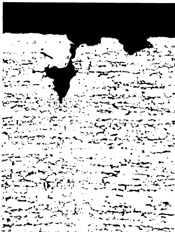
L-64-8304 Figure 10.- Pits in PH 15-7 Mo transverse specimen exposed for 7000 hours at 550° F (561° K). 500x.
