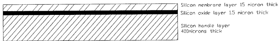
Figure 19: Cross-sectional view of an silicon-on-insulator (SOI) wafer.
