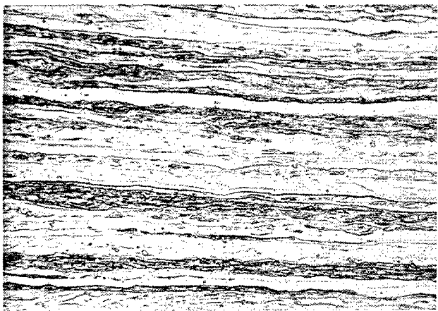
(h) Longitudinal section of 0.040-inch-thick molybdenum - 0.5-percent-titanium specimen as received. X500.
