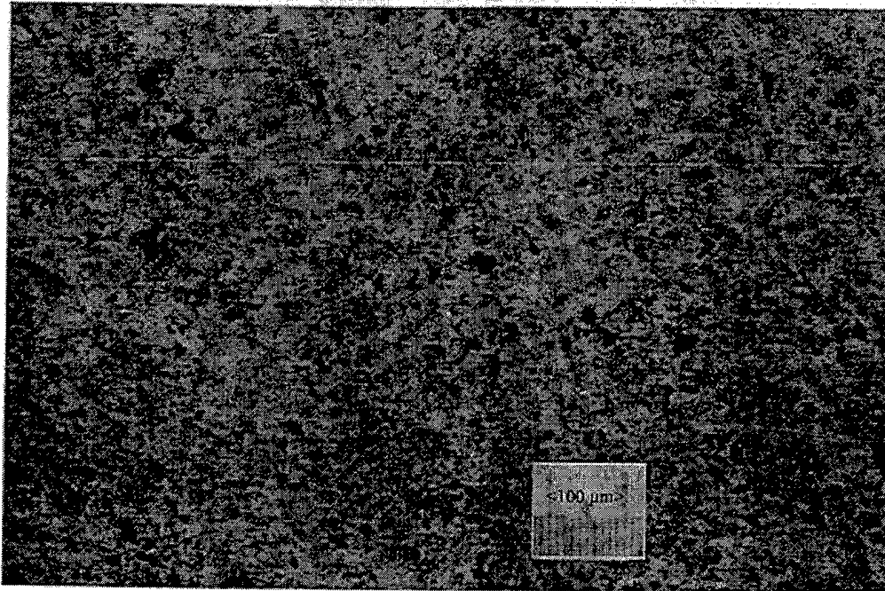
Figure 8. Optical microscope photo of a 2.5-mm-thick sheet of virgin JA2.
