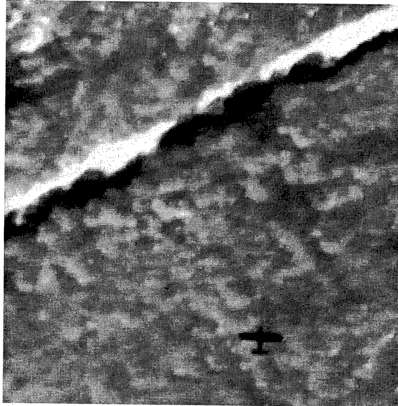
Figure 2. QWIP IR. Image of Cessna against natural background. Provided by Naval Research Laboratory.
