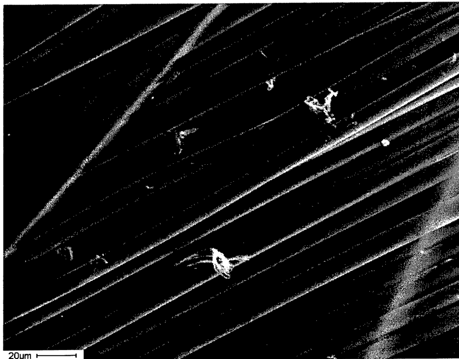
Figure 13. SEM photograph of fibers from glass fabric overwrap used on thrust chamber.
