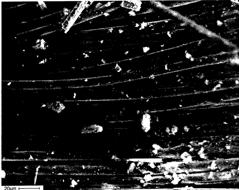
Figure 12. SEM photograph of fibers from silica phenolic liner of test fired thrust chamber.
