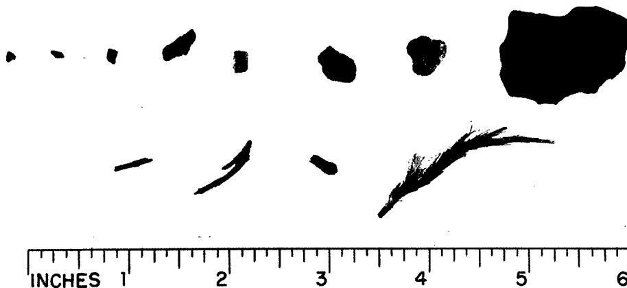
Fig. 6.1— Typical glass-fragment missiles (top row) from window panes and stone (middle row) and stick (bottom row) missiles from open areas. Glass-fragment masses, in grams (left to right): 0.0074, 0.0148, 0.0301, 0.0613, 0.1254, 0.2403, 0.5000, 1.114, 2.623, 6.840. Stone masses, in grams: 0.0063, 0.0101, 0.0142, 0.1028, 0.1059, 0.4234, 0.6719, 4.516. Stick masses, in grams: 0.0068, 0.0307, 0.0324, 0.0974.
