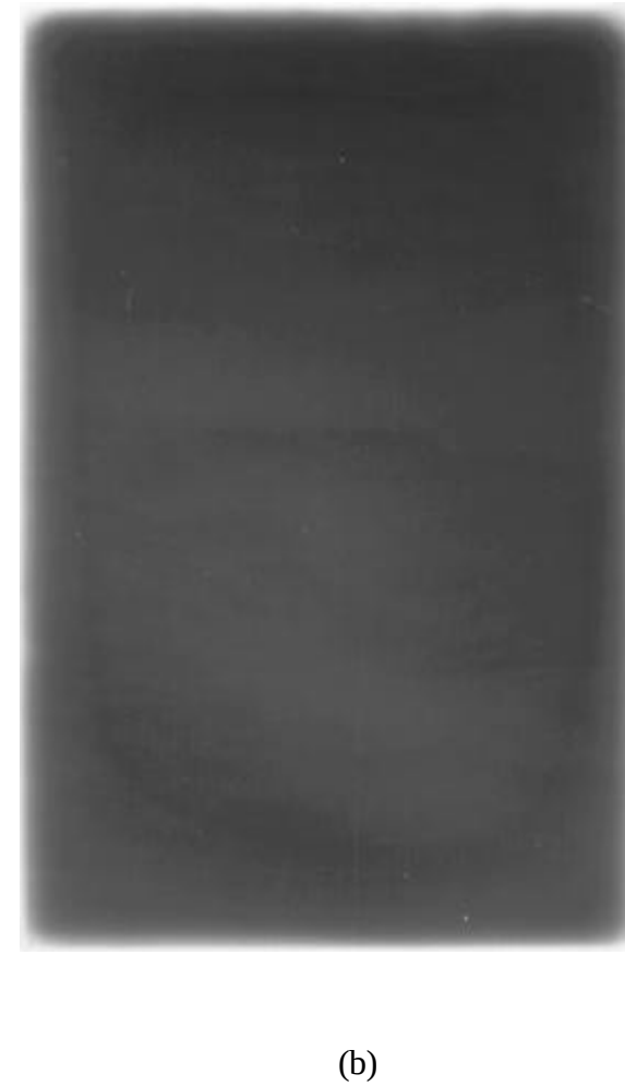
Figure 3.16 (a) & (b) X-ray radiographs of representative plates of the \text{Si}_3\text{N}_4 -BN fibrous monolith and neat \text{Si}_3\text{N}_4 materials respectively. A large number of microstructural defects are detected and the radiograph of the FM material whereas the neat material appears to be uniformly dense except near the edges.
