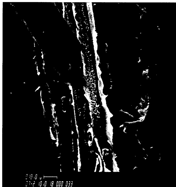
Fig. 3. Fractured surface PE/E-glass (700 ×).
