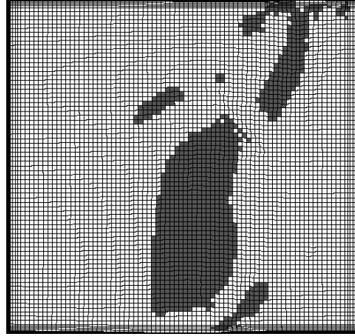
(b) Fringe plot of matrix cracking (FV1) in the bottom 45° ply
