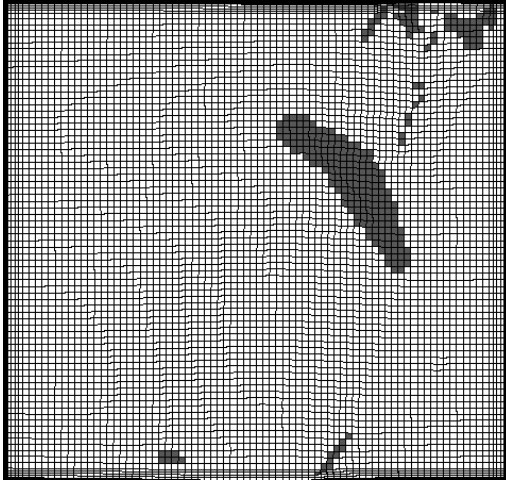
(c) Fringe plot of fiber-matrix shear failure (FV2) in the bottom 45° ply.
