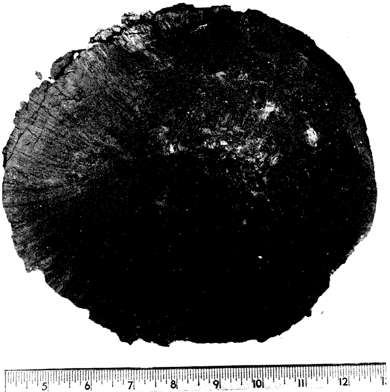
Figure 64c. Plan View of Soil Nose Taken from 9-inch Blunt Nosed Projectile After Penetration Into Playa
