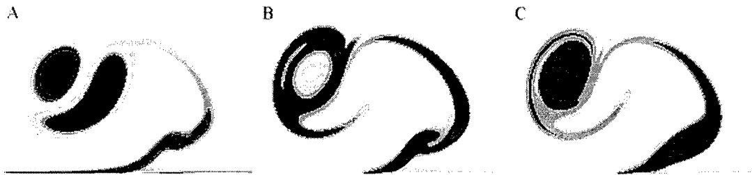
Fig.5. Fragments of vorticity and eddy viscosity fields for turbulent flow, T=4 , Re=3 \times 10^6 . A - vorticity field, SARC model, B - eddy viscosity field, SARC model, C - eddy viscosity field, SA model.
