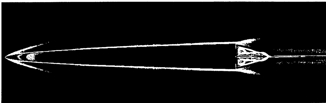
Figure 15. CFD results for zero alpha, Mach 4.2, free-flight conditions - surface colored by pressure, Schlieren on the symmetry plane, and streamlines in the base region
