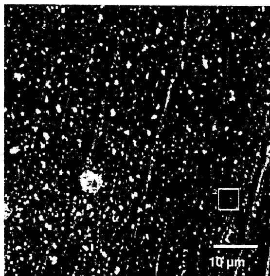
Figure 9. Backscatter scanning electron micrograph of a 6061-T6 surface exposed in the simulated scratch cell for 48 hours to 0.5 M NaCl. The other surface exposed in the cell was Ce-modified hydrotalcite. Two analysis regions are indicated. Region 1 is on a deposit located over a Cu-rich particle. Region 2 is on the matrix phase.
