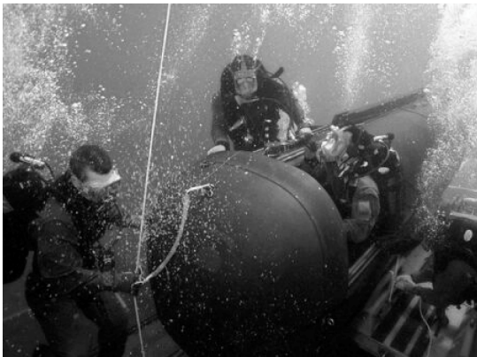
(left) The SEAL Delivery Vehicle has limited endurance, wet compartments, and can operate in shallow water.
