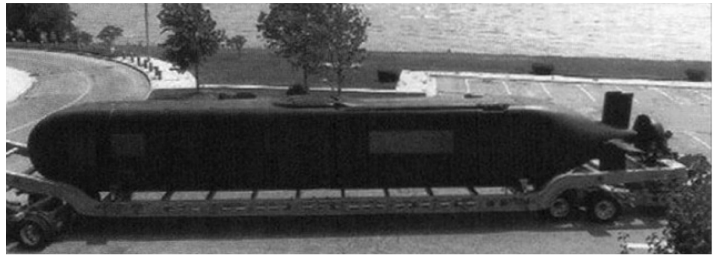
(left) The SEAL Delivery Vehicle has limited endurance, wet compartments, and can operate in shallow water.
