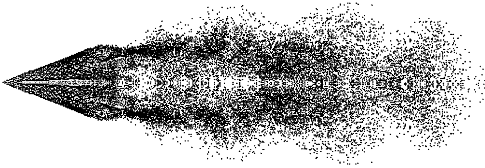
Figure 7 Top view of vortex wake past delta wing with twin tails at 40 degrees angle of attack
