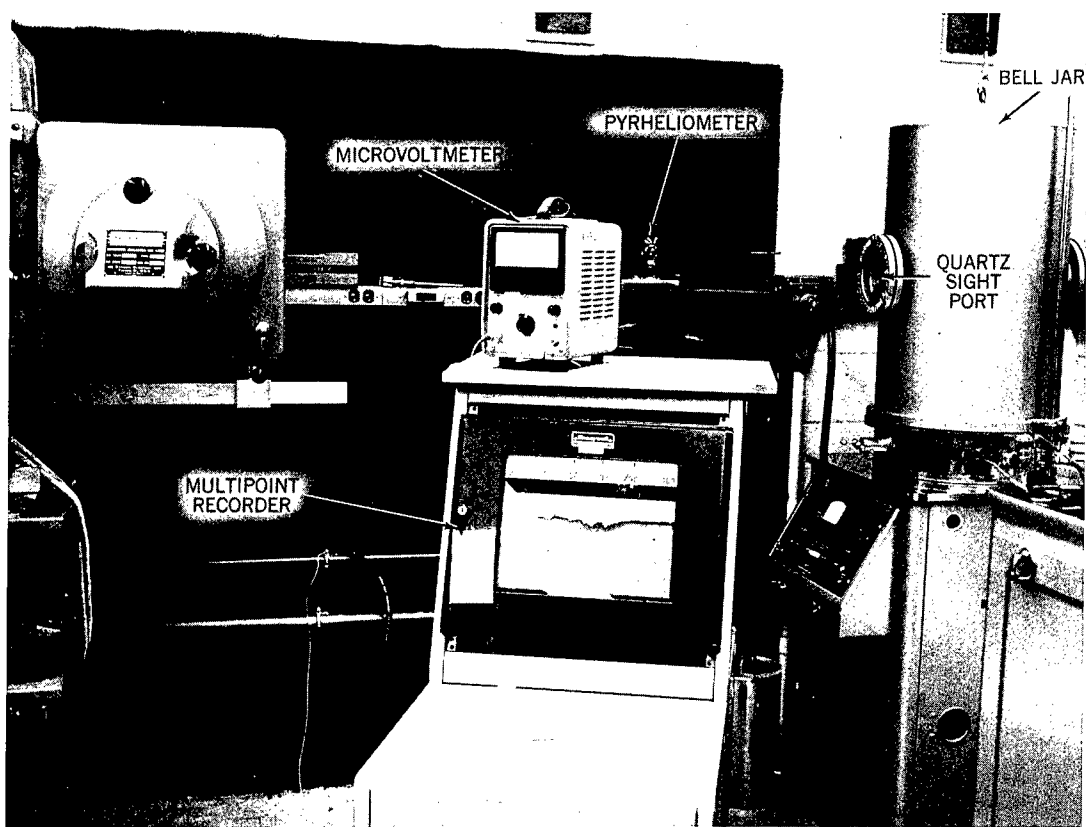
Figure 4—The complete thermal vacuum setup showing solar simulator (carbon arc), light intensity measuring equipment, and multichannel temperature recorder. Bell jar is in the "operating" position.
