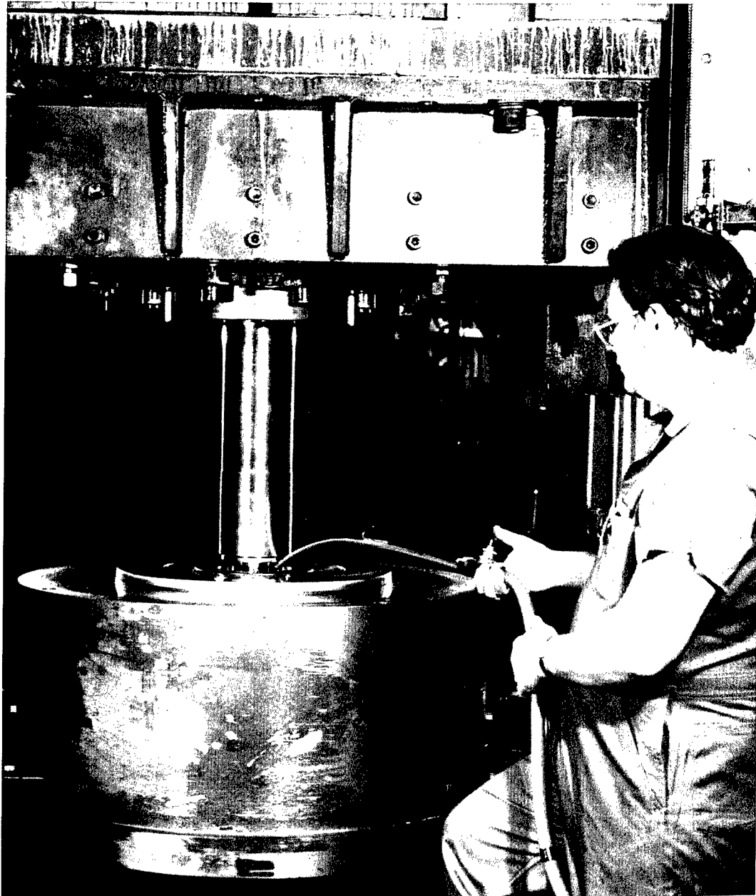
FIGURE 18. INJECTION OF HYDROSTATIC FLUID INTO HYDRAFILM EXTRUSION CONTAINER
