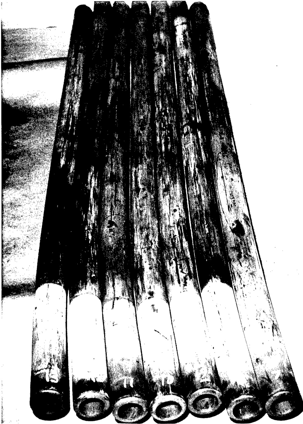
FIGURE 23. AS-EXTRUDED 4340 STEEL TORSION TUBE BLANKS FORMED IN SECOND SERIES OF TRIALS
