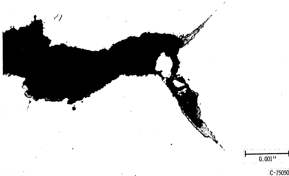
Figure 12. Evidence of blunting of crack tip by oxide in Inconel 550 specimen fatigue tested for 1366 hours. Ratio of cyclic to mean stress, 0.667. X750.
