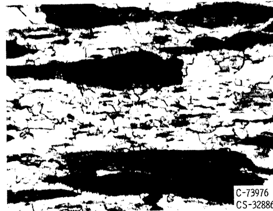
Figure 1. - Continued. Microstructures of as-extruded tungsten and tungsten-oxide composites. X500. (Reduced 30 percent in printing.)
