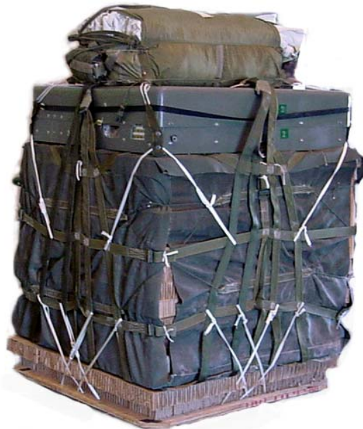
Figure 3.13 Serial/Autonomous AGAS package rigged for deployment
