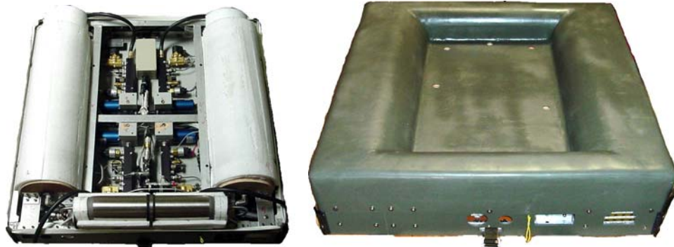
Figure 3.14 Serial/Autonomous AGAS package open and top views
