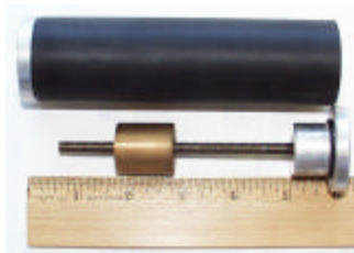
Figure 3. Internal Components of Mine Shape
