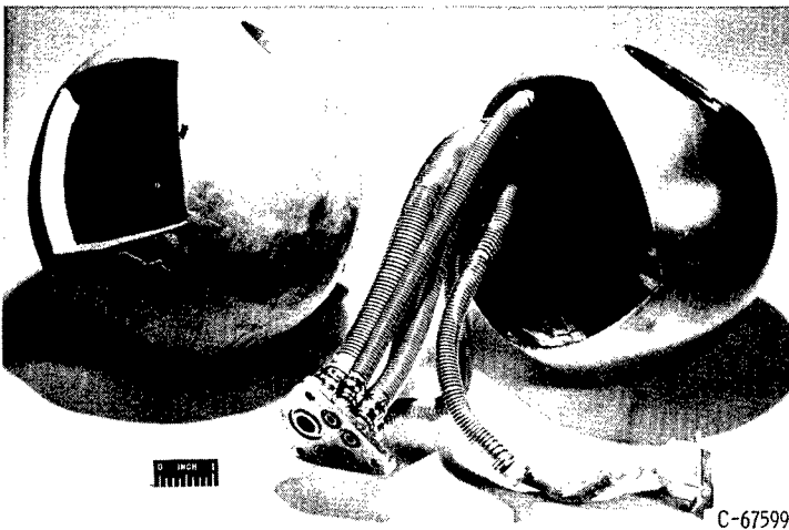
Figure 10. - Nose instrument housing of X-15 airplane.
