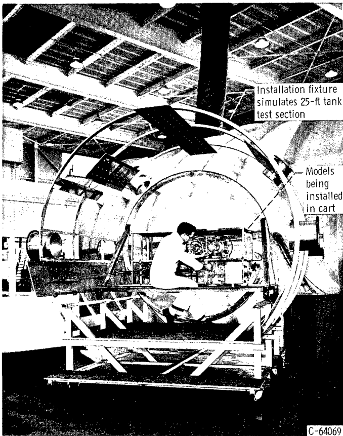
Figure 10. - Thrustor installation in cart and installation fixture.
