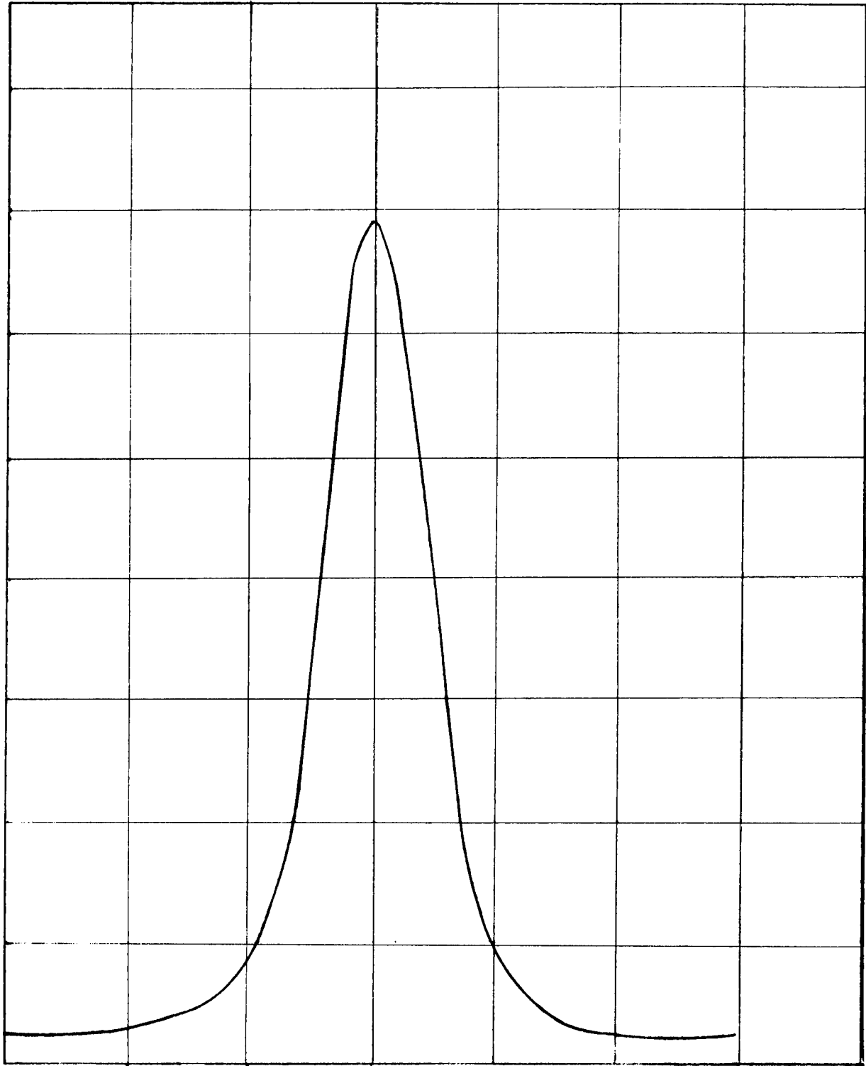
Figure 14. The 200 x-ray diffraction line obtained from cold worked pure nickel
