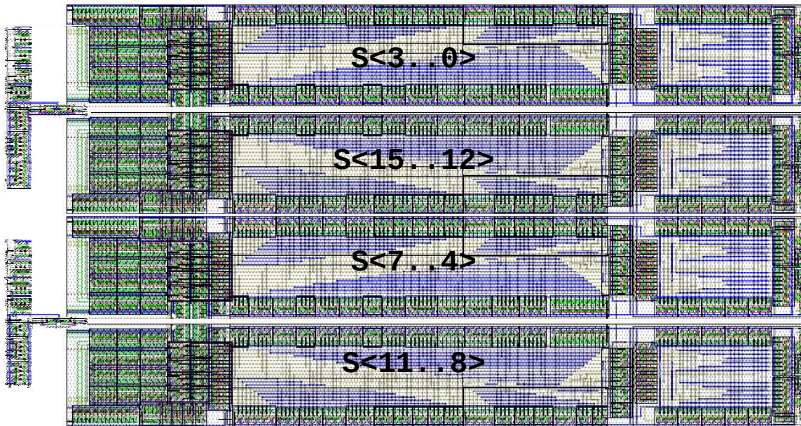
Figure 37. Integration of CLAH in 16-Bit Adder.
