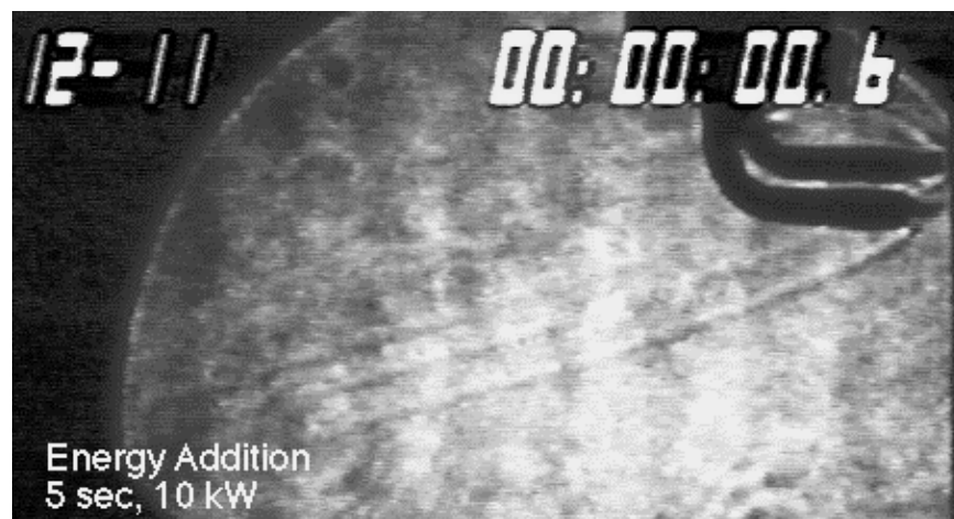
Figure 7-4b. Shadowgraph of flow around pitot pressure and total temperature probe at the nozzle exit with energy addition . Flow is again from right to left. A comparison between the Mach angle of Figs. 7.4a and 7.4b shows a decrease in Mach number from 4.2 to 3.9.
