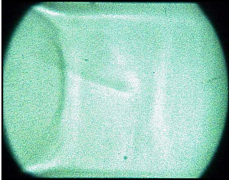
Figure A.8. Normal shock resulting from sting mount blockage using Mach 1.7 nozzle blocks with 50 psig plenum pressure and relief valves closed.
