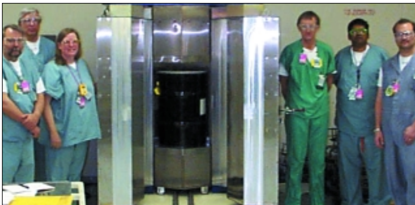
Experimental test measurements of plutonium-bearing weapons components using neutron multiplicity counting at the Rocky Flats Environmental Technology Site.
