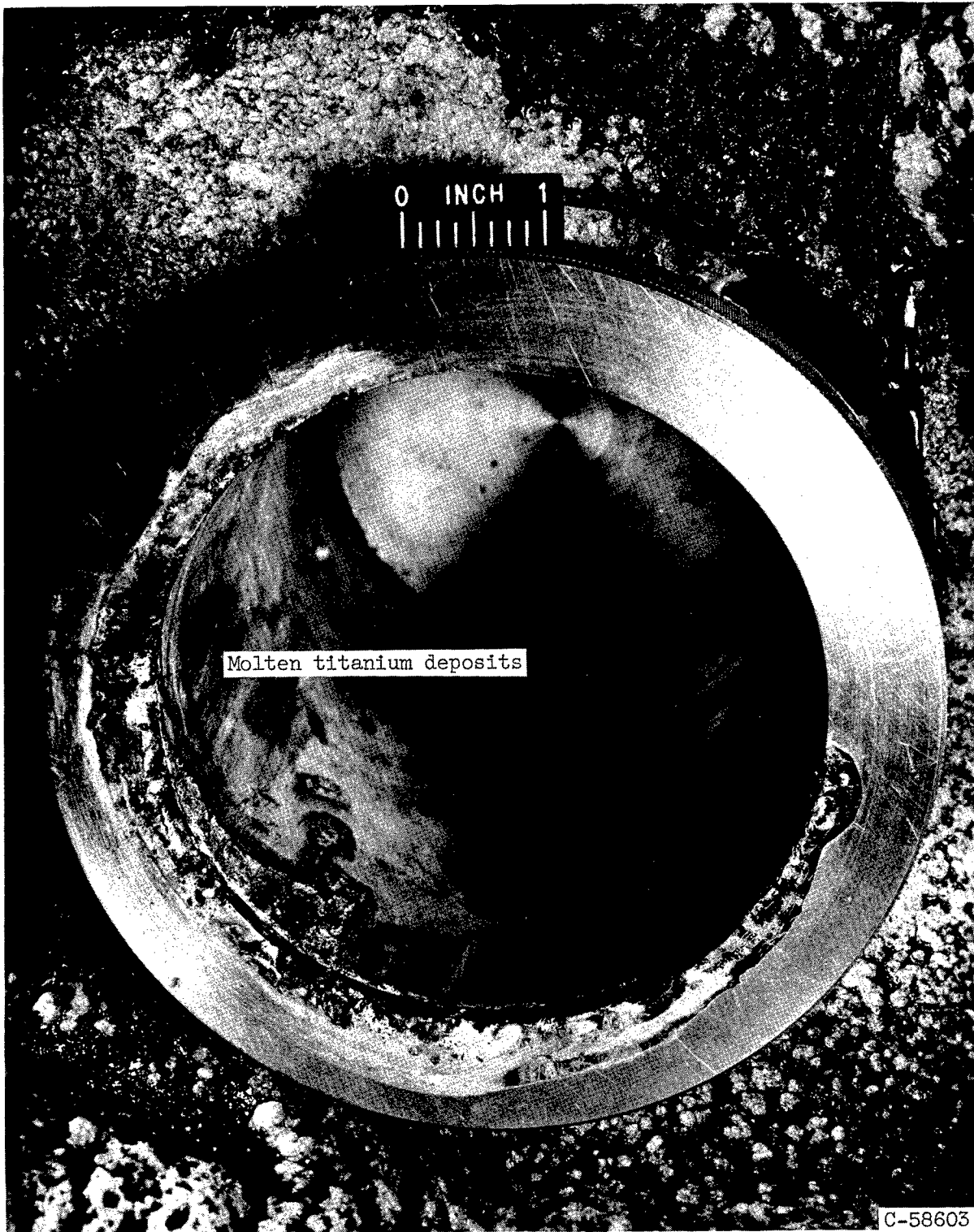
Figure 12. - Condition of tank after impact and penetration of titanium wall of tank filled with liquid oxygen. Test 8.
