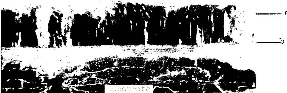
(c) Cross section, polarized light. X500.
