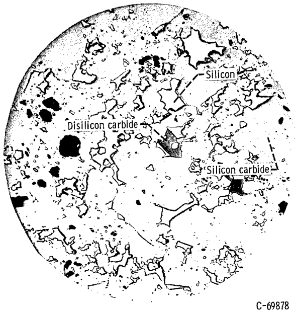
Figure 1. - Microstructure of self-bonded silicon carbide ball specimen. X140.
