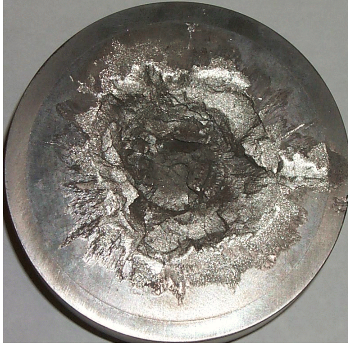
Figure 3. \text{TiB}_2 disk with prestress; single impact.
