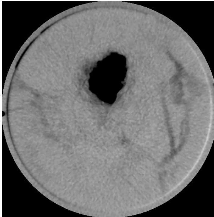
Figure 25. CT slice 23.5 mm from impact face of the TiB 2 disk used in test no. R-1 (2nd).
