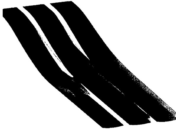
Figure 6.21: 3-D steady RANS. Corrugated surface. Isocontours of \omega_x = 0.002 (green), w = -0.0005, 0.0005 (red, blue), and u = 0.737 (cyan).
