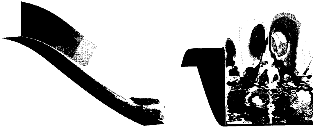
Figure 2.6: POD of 3-D DNS, mode 0. Isosurfaces of u = 0.5 (cyan), w = -0.01, 0.01 (red, blue), isocontours of u (left), and isocontours of w (right).
