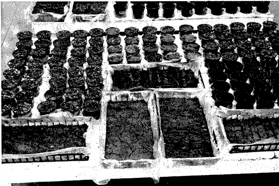
Figure 10. Overall view of the seed germination test using dredged material from Toledo Harbor Cell 1 CPF as the primary ingredient in the manufactured topsoil blends
