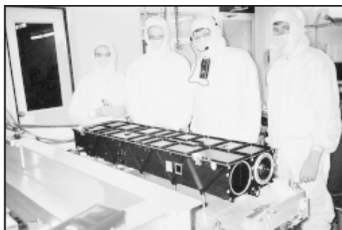
French and English colleagues assist NRL scientists preparing the LASCO wide-field coronagraph for flight on SOHO
