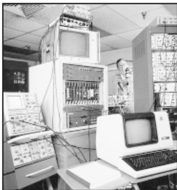
The Focal Plane Array Evaluation Facility consists of the optical sources and electronics required to evaluate monolithic or hybrid infrared focal plane arrays that use charge-coupled device, charge-injection device, direct readout, or charge-imaging matrix technologies
