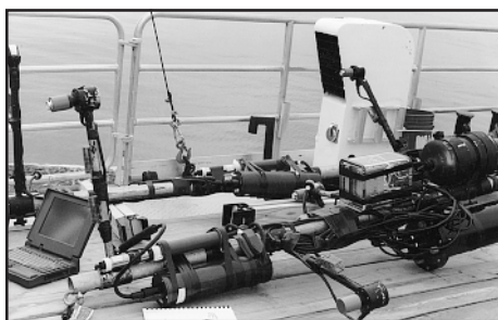
Optical mooring equipment for shallow water showing attenuation and absorption meters and irradiance sensors
