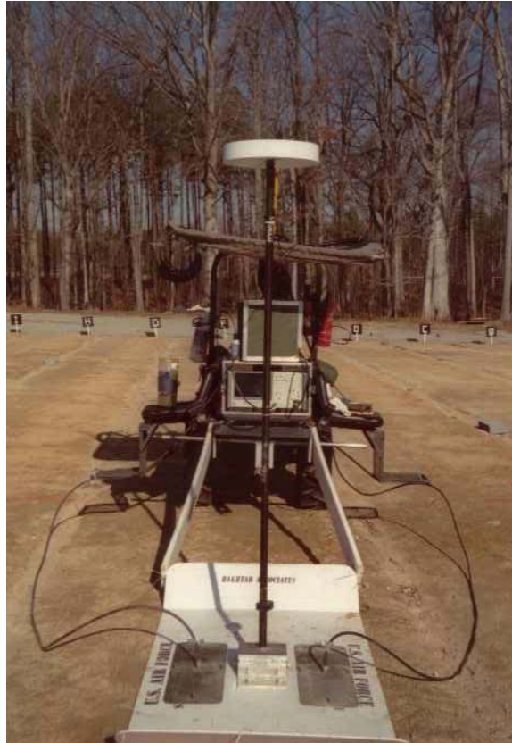
Figure 2. Photograph of Typical EarthRadar Antennas
