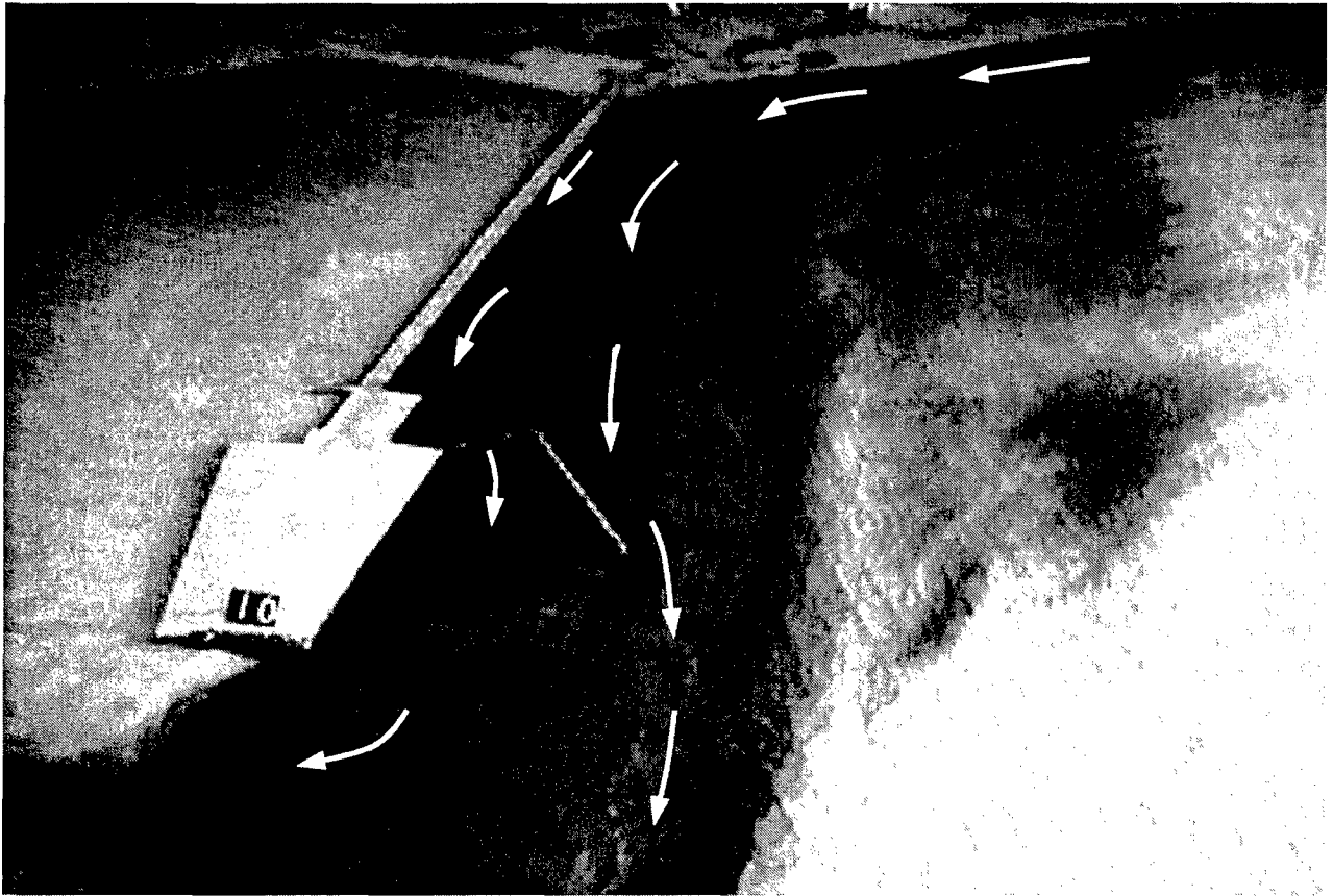
Photo 9. Typical wave and current patterns for existing conditions; 2.7-sec, 0.4-m (1.3-ft) waves from 90 deg
