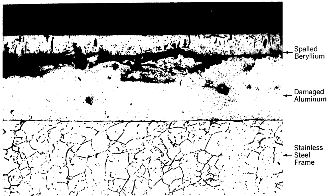
Figure 6—Photomicrograph (500X) beyond ultrasonic weld, showing foil damage. Stainless steel frame etched electrolytically in 10 percent oxalic acid. Beryllium etched in 10 percent HF, 90 percent ethanol.
