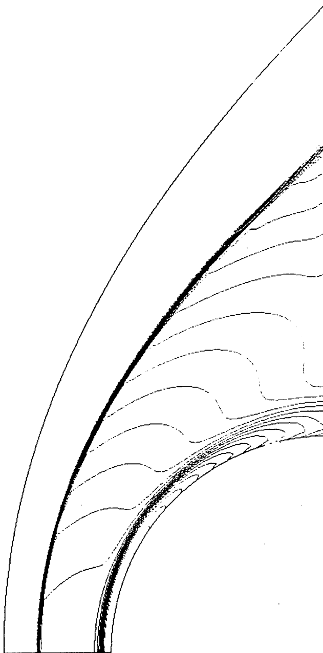
Figure 36: Temperature contours: M = 6.61 methane/air, 1 mm diameter. Contour levels: min: 250 K, max: 3130 K, inc: 93 K.
