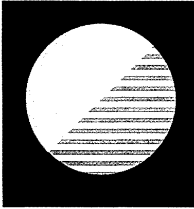
Figure 6. The disk pattern for estimating the CRT gamma.
