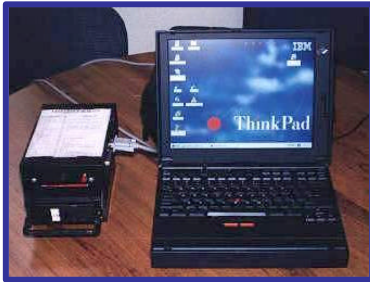
Figure 4. Typical PFPS System for F-16 mission planning. 3
