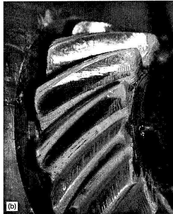
Figure 6.—High load contact patterns for gears. (a) Face-milled. (b) Face-hobbed.
