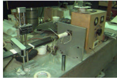
Test 2 SMA Torque Tube Shown in Test Rig
