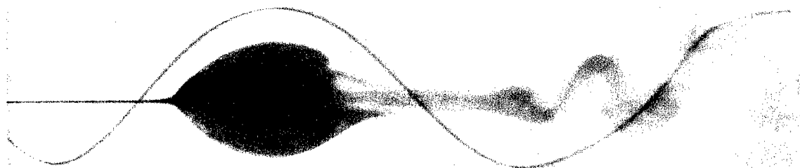
Figure 1-6, Vortex breakdown in a pipe ( ref. 8 )
