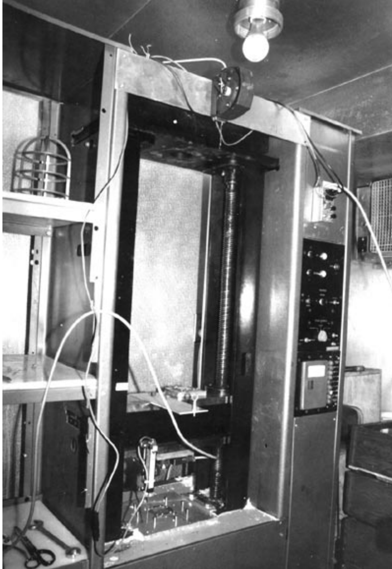
Figure 4. Instron Universal Testing Instrument used for compressive strength tests. The bottom platen is shown in place while the top platen is lying on top of the press head.
