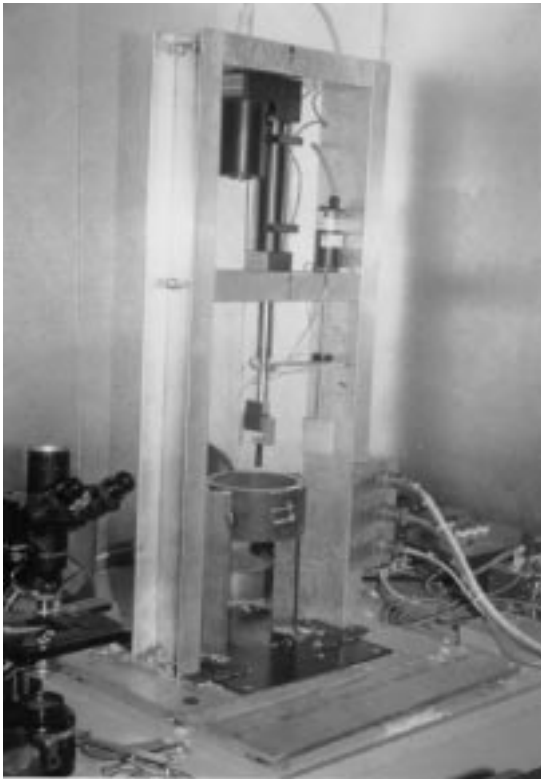
Figure 8. CRREL snow load frame used for flexural strength testing. The sample disk was placed across the metal cylinder centered beneath the indenter.
