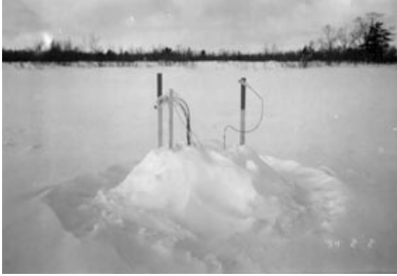
Figure 10. Snow mound enclosing the stack of 12 sample bricks used to study the effect of a thermal gradient on CFG ice. The cluster of wires on the left lead to the 12 thermocouples embedded in the stack. The single lead on the right leads to a thermistor probe installed about 10 cm from the stack. Plastic bags cover the connectors for all of these leads.
