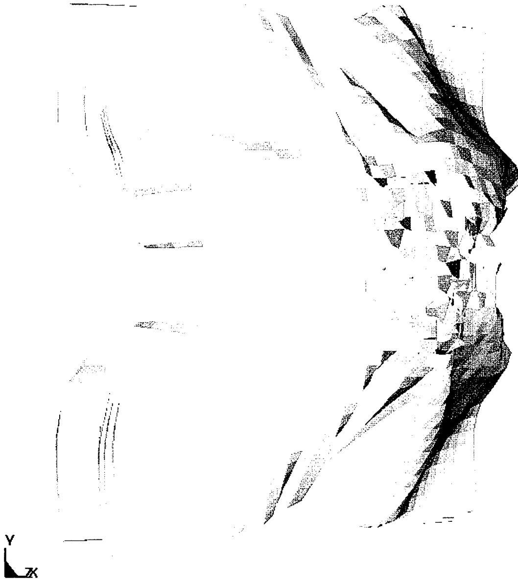
Figure 3. LS-DYNA simulation at 70 \mu s into run showing damage up to the fifth ply ( V_s = 200 m/s).
