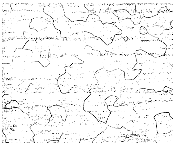
Figure 35. Longitudinal Microstructure of V-20w/oTi Cold-worked 25% and Vacuum-annealed for 1 hr at Various Temperatures (Etchant: 5% HF, 2% AgNO 3 )
