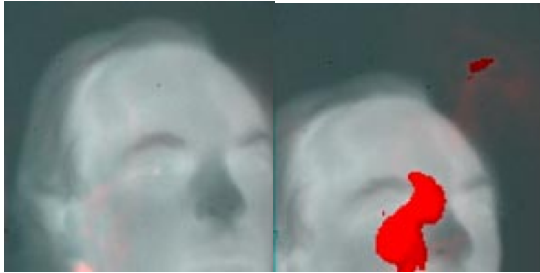
Figure 17a & b Highly correlated image with weak MW2 signal before and after difference/threshold process
