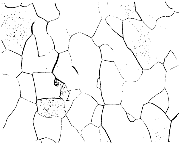
(c) Annealed for 1 hour at 2400° F; fully recrystallized; average grain diameter, 0.0211 centimeter.
